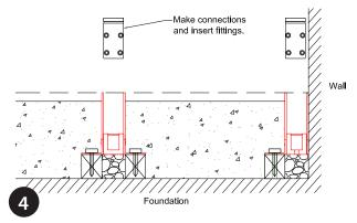
Make product power connections ensuring they are appropriate for the environment, pack cables into housing ensuring that no stress or pinching occurs as product is fitted into housing. Ensure product is pushed fully into housing clips.
