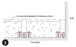
Ensuring housing end caps and housing cover is installed, pour concrete or floor material as required. If finished floor is tiled, grout or mastic can be used to fill gap between housing and finished floor. Ensure that adequate drainage is allowed.
